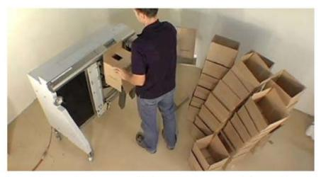
A revolutionary simple answer for tape erecting cases. Ergonomic waist high forming, cases are delivered back into the packers hands.
