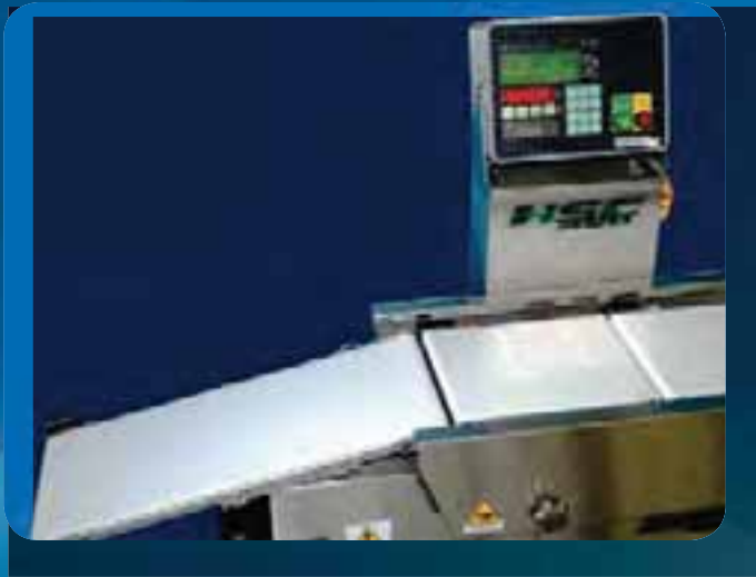
Fall conveyor rejector
