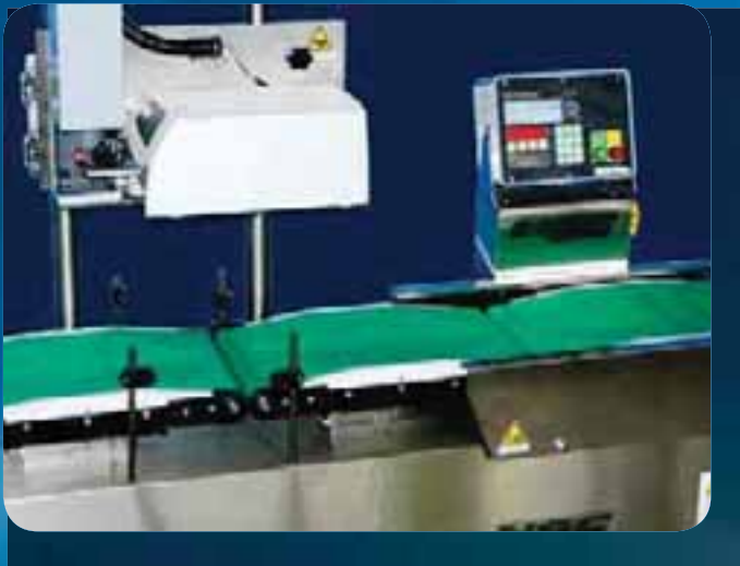
Top label application with special conveyor for round product
