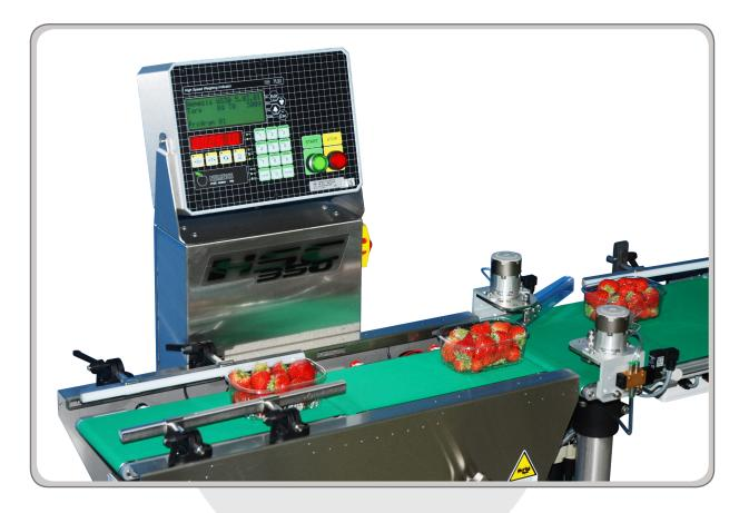
The HSC350 Serie "Z" is an high speed checkweigher for small packages (punnets, chests, cans, small trays, ... ) integrated with a sorting system capable of splitting product in up to three channels, usually divided as underweight, complying and overweight.
